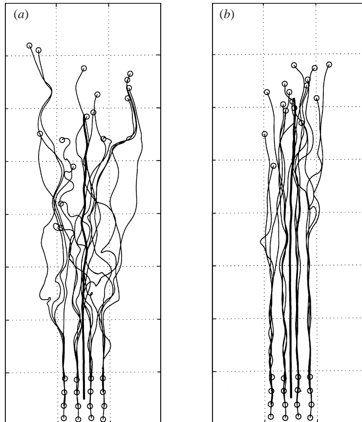
FIGURE 3. The path of the individual bubbles in the simulation in figure 2 is shown on the left ( a ) and the path of bubbles computed by neglecting all inertial effects (Stokes flow) is shown on the right ( b ). The bubbles originally in the computed period are followed as they rise through the other periods. The horizontal and vertical dashed lines mark the boundaries between successive periods. The thick, solid line marks the motion of the centroid of the bubbles. Notice that the small circles that mark the beginning and the end of each path are much smaller than the bubbles.
